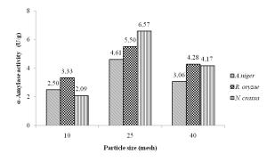
Figure 2. The effect of particle size on the α-Amylase activities, which was measured after 5 days incubation at 30°C
