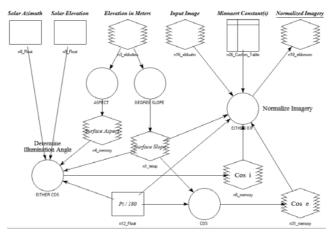
Figure 2.. Topographic normalization process (ERDAS Imagine).
